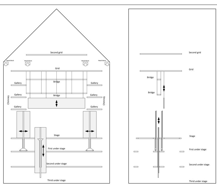
blocks on the outside, go up and down. On the inner (stage) side, pin rails are placed to fix ropes coming from the head blocks on the grid. Additional winches are placed on different points to be able to pull up the counter weights. be pretty full as sets for several performances can be in place at the same time. During movements they have to be kept apart to avoid damage.
