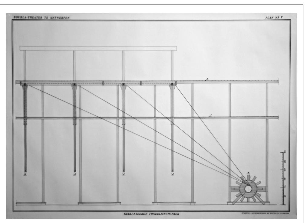
connected that runs into a slit along the batten. The cassette contains sheaves that change the direction of the rope in order to manipulate the height of the batten and to connect counterweights.
