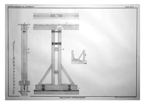
A post is mounted on the chariot to fix a flat on. The post will pass from the under stage to the stage through the costieres. In modern theatre the portal towers making the stage less wide are still constructed by this principle. In cases where the flats had to turn, a turning post was used, the "Chasis obliques"
