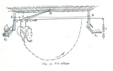
The control rope holds the wagon in place. Slackening the rope makes the object go in a curve with the lowest point under the fixed point. In modern theatre this movement is controlled differently now. By using a double sheave system the vertical movement is not influenced by the horizontal movement.
