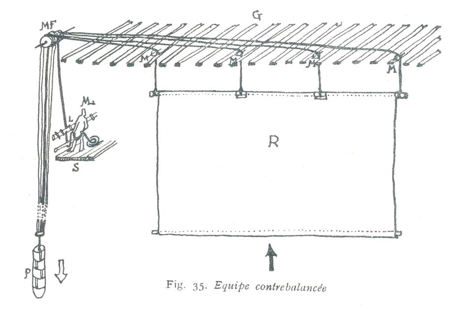
As there are only ropes where needed, flats hung on the sides don't impede movements in the middle. This makes it for example possible to have a fly rail from front to back stage.
